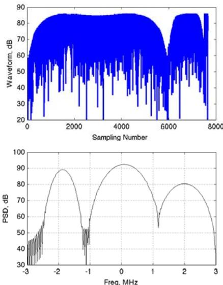
Figure 5. An example of the three-pulse TFM waveform (upper row) and its spectrum (lower row)
