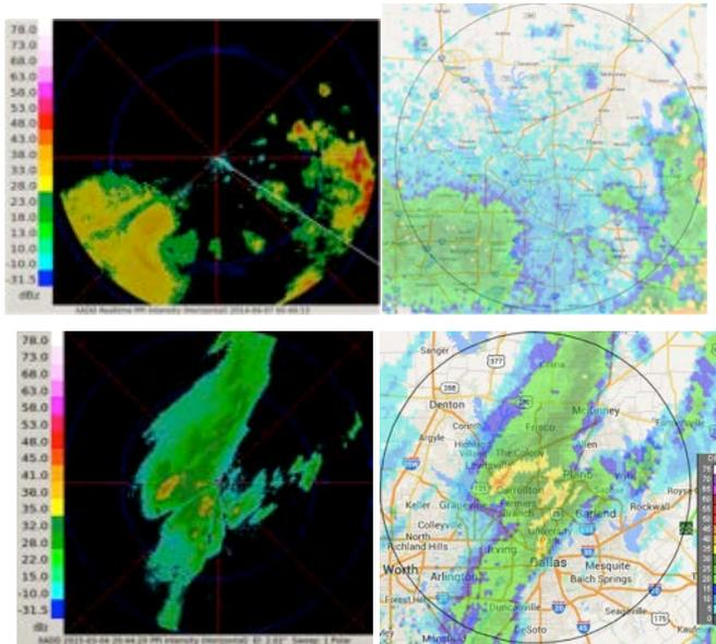
Figure 9. Comparison of reflectivity measurements from Ranger-X1 (left) and NEXRAD KFWS radar (right).
