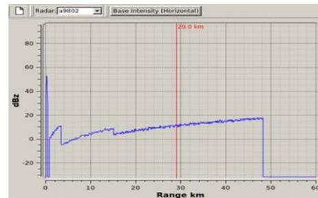
Figure 7. The sensitivity of Ranger-X1 shown in the EDGE A-scope display of base reflectivity
