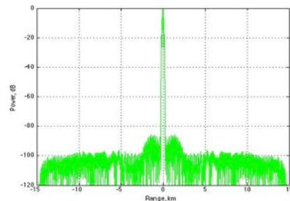
Figure 6. The theoretical range sidelobe pattern for one of NLFM waveform designs.
