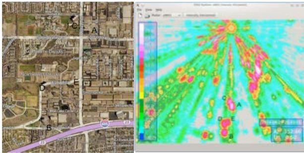
Figure 8. Example of clutter measurements used for the calibration of antenna azimuth angle.
