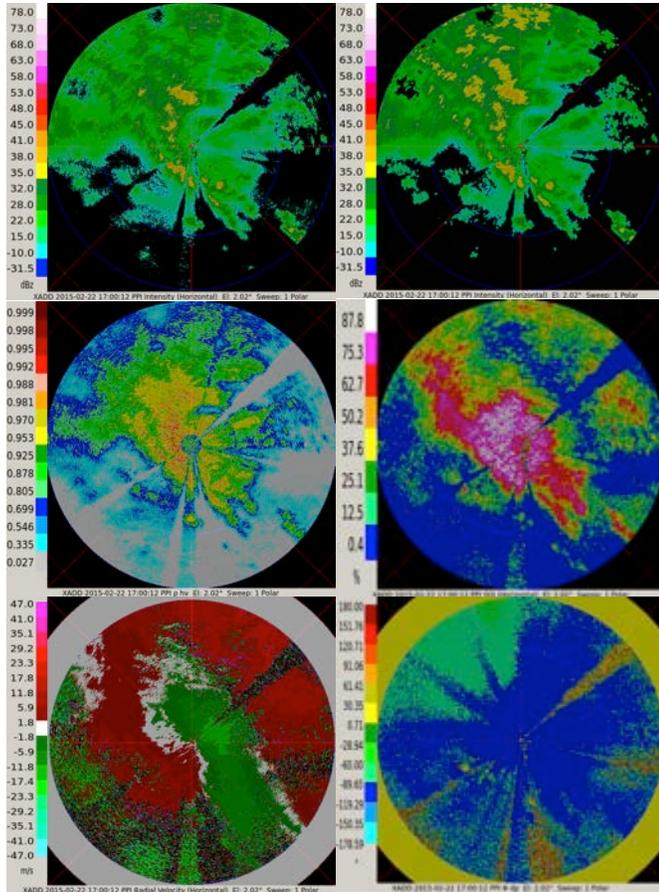
Figure 11. Ranger-X1 measurements (from top to bottom, left to right): raw  $Z_H$ , corrected  $Z_H$ ,  $\rho_{hv}$ , SQI,  $v_h$ , and  $\Phi_{dp}$ .
